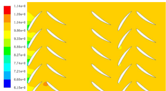
Fig. 16 Static pressure distribution when removing the entire rotor blades of the middle stage
