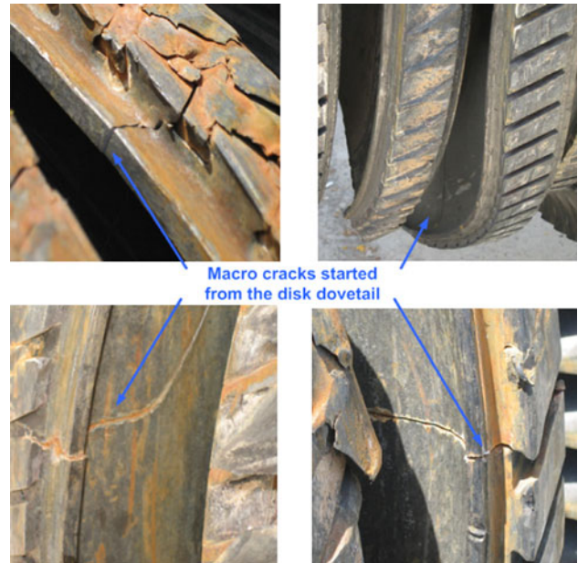
Fig. 4 Cracks initiated from the dovetail regions on the compressor disks and propagated toward the disks body [16]
