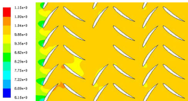
Fig. 18 Static pressure contours when removing only two rotor blades of the middle stage
