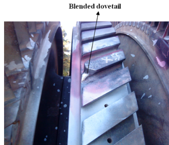
Fig. 8 A blended dovetail of the damaged disk of stage 11
