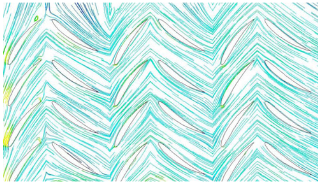
Fig. 13 Stream lines in complete cascade
